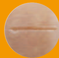
Super-Pulse mode pulse duration=10µs
